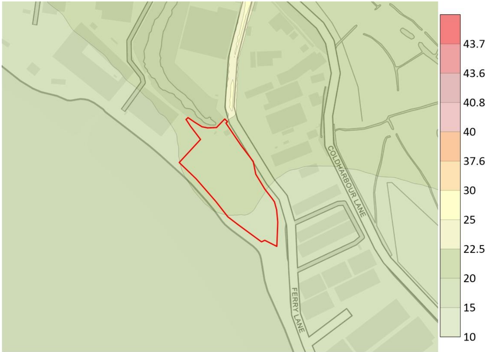
Figure 5-2. Total Long Term Annual Average Nitrogen Dioxide (NO 2 ) Concentration at Proposed Development (µg/m 3 )
